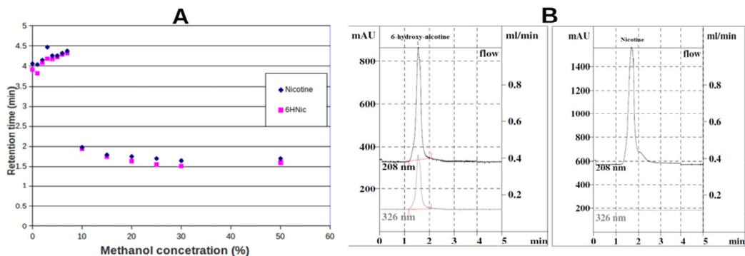
**Figure 1. A.** Dependence of nicotine and 6-hydroxy-nicotine retention times on the methanol concentration. Largest differences in retention times were obtained at a methanol concentration of 25%. **B.** Typical HPLC run for separation of nicotine and 6-hydroxy-nicotine using 1mN H<sub>2</sub>SO<sub>4</sub> : methanol 75:25 as mobile phase.
