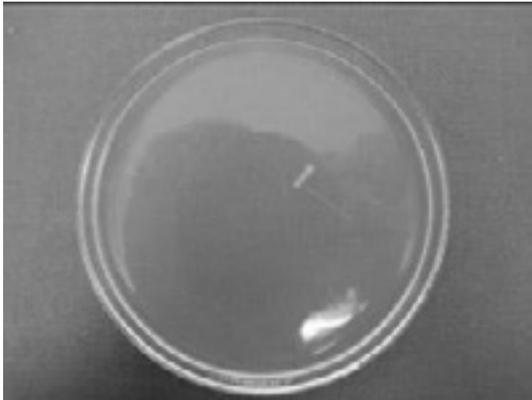
Photo 3 - Microbial load of sample P2 before processing with brushes and polishing paste that had not been used before (dilution  $10^{-3}$ )
